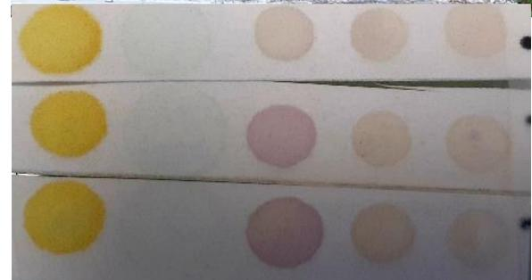
Top: testing the sensor array in the brood of a healthy hive. Bottom: colourimetric sensor strips used in B-CHECK
